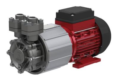
These non-self-priming regenerative turbine pumps with magnetic coupling are characterised by high pressure at low flow rates and a compact construction. Thanks to the magnetic coupling they are leakage and maintenance-free. They can be applied in circuits for liquids not containing solid matter, for example in cooling circuits or in temperature control units, among others.
