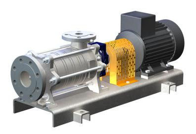
These self-priming, gas handling side channel pumps have a very low NPSH level, thanks to the NPSH suction level, which is why they are used for applications in which there are difficult suction or intake conditions, for example in boiler feed pumps or condenser pumps.
