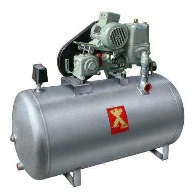
The pump, which is assembled on site, is type tested and consists of the following parts: Pumpmeister piston pump with built in membrane safety valve (type tested), electric motor, galvanized pressure vessel, pressure switch programmed from 0.2 to 3.5 bar, pressure gauge, ventilation machine, completely closed belt guard made from plastic for your safety. A motor protection switch must be provided on site.
