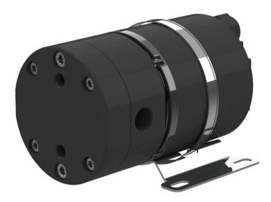
These self-priming gear pumps with electronically commutated direct current motor, in a canned motor version, are maintenance-free and can be set to various motor speeds. These can be applied for example in medical technology and fuel delivery.
