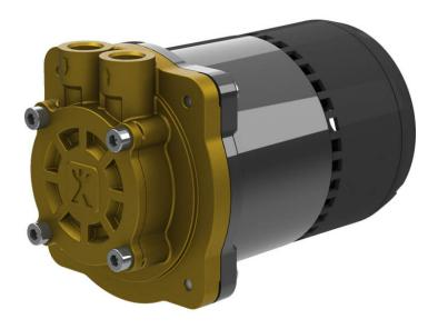
These non-self-priming regenerative turbine pumps with electronically commutated direct current motor, in a canned motor version, are maintenance-free and can be set to various motor speeds. These can be applied for example in temperature control technology and in industrial cooling.
