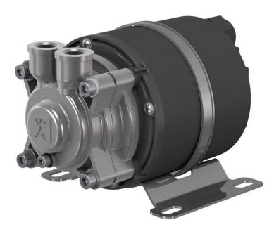
These non-self-priming regenerative turbine pumps with electronically commutated direct current motor, in a canned motor version, are maintenance-free and can be set to various motor speeds. These can be applied for example in temperature control technology and in industrial cooling.
