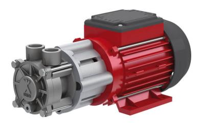
These non-self-priming regenerative turbine pumps with magnetic coupling are characterised by high pressure at low flow rates and a compact construction. Thanks to the magnetic coupling they are leakage and maintenance-free. They can be applied in circuits for liquids not containing solid matter, for example in cooling circuits or in temperature control units, among others.
