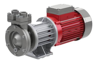
These non-self-priming regenerative turbine pumps with magnetic coupling are characterised by high pressure at low flow rates and a compact construction. Thanks to the magnetic coupling they are leakage and maintenance-free. They can be applied in circuits for liquids not containing solid matter, for example in cooling circuits or in temperature control units, among others.
