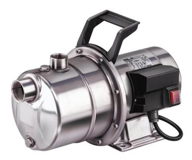
All wetted parts in the SG/SGM self-priming centrifugal pump range are corrosion-resistant. The motor bearings are lubricated for life. The maintenance-free mechanical seal is designed for continuous operation. The single phase version SGM is fitted with an on/off switch in the terminal box as well as a 1.5 m cable with a shock proof plug.
