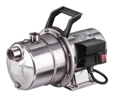
All wetted parts in the SG/SGM self-priming centrifugal pump range are corrosion-resistant. The motor bearings are lubricated for life. The maintenance-free mechanical seal is designed for continuous operation.
