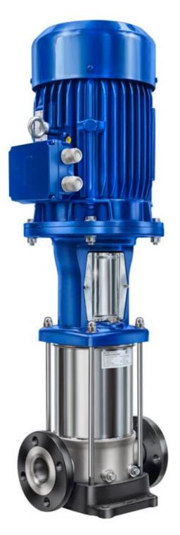
Vertical, multistage centrifugal pumps from the IN-VB range are non-self-priming high pressure pumps characterized by a high rate of efficiency as well as durability. Wetted parts are made from AISI 304 or AISI 316 L stainless steel. The ? 0.75 kW three-phase motors correspond to the energy efficiency classification IE3.
