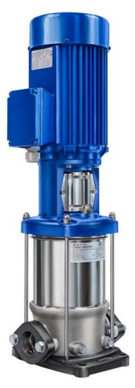
Vertical, multistage centrifugal pumps from the IN-VB range are non-self-priming high pressure pumps characterized by a high rate of efficiency as well as durability. Wetted parts are made from AISI 304 or AISI 316 L stainless steel. The ? 0.75 kW three-phase motors correspond to the energy efficiency classification IE3.
