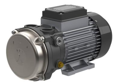
These liquid ring vacuum pumps are single-stage pumps with an internal water restraint system. The water-saving and low-noise construction, as well as a low susceptibility to calcification, is some of the benefits. These pumps are applied in small sterilisers and degassing units, among others.
