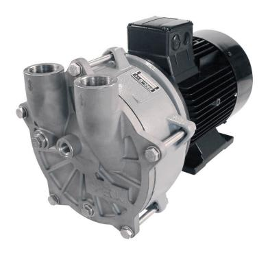
These liquid ring vacuum pumps are single-stage pumps without valve flaps. Thanks to their construction with almost no dead space, they are also suitable should there be any contamination in the media. These pumps are applied in sterilisers, degassing units and plastic extrusion, among others.
