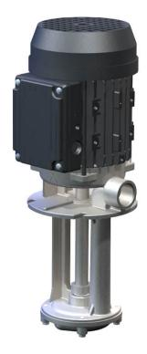
These submersible pumps with peripheral impellers are characterised by their high pressure and their sealless, low-maintenance construction. They can be applied in circuits with media not containing solid matter, for example in temperature control units or machine cooling systems.
