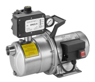
The control unit switches the pump on when the pressure is less than 2.2 bar and turns the pump off when it reaches the end pressure, runs dry or when the consumption is less than 0.6 l/min. The starting pressure cannot be changed. There must be a minimum pressure difference of 0.7 bar between the starting and cut-out pressure.
