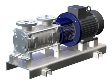
These self-priming, gas handling side channel pumps and side channel pumps with magnetic coupling handle liquids not containing solid matter and can be used for hot water applications or applications with great suction heights, for example boiler feed pumps or condenser pumps. Due to the magnetic coupling there is no shaft seal and the pumps can therefore also be used for difficult media.
