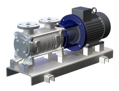
These self-priming, gas handling side channel pumps and side channel pumps with magnetic coupling handle liquids not containing solid matter and can be used for hot water applications or applications with great suction heights, for example boiler feed pumps or condenser pumps. Due to the magnetic coupling there is no shaft seal and the pumps can therefore also be used for difficult media.
