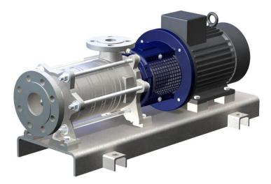
These self-priming, gas handling side channel pumps with magnetic coupling have a very low NPSH level, thanks to the NPSH suction level, which is why they are used for applications in which there are difficult suction or intake conditions, for example in boiler feed pumps or condenser pumps. Due to the magnetic coupling there is no shaft seal and the pumps can therefore also be used for difficult media.
