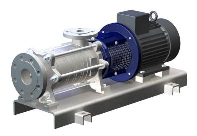
These self-priming, gas handling side channel pumps with magnetic coupling have a very low NPSH level, thanks to the NPSH suction level, which is why they are used for applications in which there are difficult suction or intake conditions, for example in boiler feed pumps or condenser pumps. Due to the magnetic coupling there is no shaft seal and the pumps can therefore also be used for difficult media.
