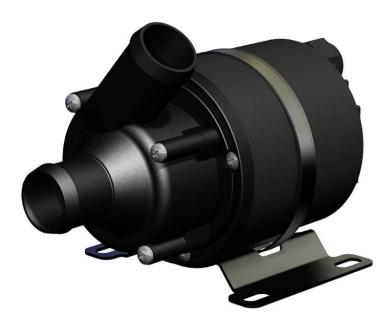
These non-self-priming centrifugal pumps with electronically commutated direct current motor, in a canned motor version, are maintenance-free and can be set to various motor speeds. These can be applied for example in cooling circuits and in air-conditioning units in cars.
