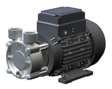
These non-self-priming regenerative turbine pumps are characterised by high pressure at low flow rates and a compact construction. They can be applied in circuits for liquids not containing solid matter, for example in cooling circuits or in temperature control units, among others.
