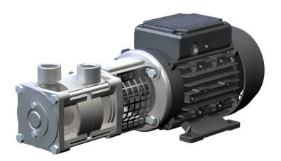
These self-priming regenerative turbine pumps are characterised by their high pressure at low flow rates and their compact construction. They can be applied in circuits for liquids not containing solid matter, for example in cooling circuits and back feeds.
