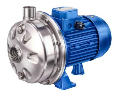
Centrifugal pumps in the VGX/2 VGX range are single and multistage pumps in a monoblock design. The non-self-priming centrifugal pumps are charaterised by a compact construction and durability. Wetted parts are made from stainless steel 1.4301.
