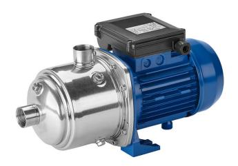
Monoblock pump with surface-cooled motor, extended motor shaft to accommodate the impellers, shaft seal in the form of a mechanical seal, configured for constant operation.
