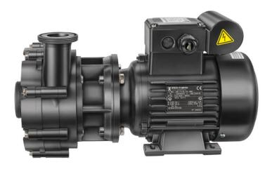
The special version AK pumps correspond to the standard versions in our BADU programme, however they are designed for use in diverse salt water and problem medias. Media that could potentially leak or minerals and salts which could crystallise do not come into contact with the motor or bearings. Therefore this ensures considerably longer operating times for these fields of application compared to the standard version.
