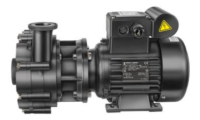
The special version AK pumps correspond to the standard versions in our BADU programme, however they are designed for use in diverse salt water and problem medias. Media that could potentially leak or minerals and salts which could crystallise do not come into contact with the motor or bearings. Therefore this ensures considerably longer operating times for these fields of application compared to the standard version.
