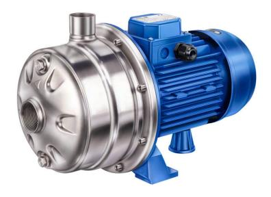
Centrifugal pumps in the VGX/2 VGX range are single and multistage pumps in a monoblock design. The non-self-priming centrifugal pumps are charaterised by a compact construction and durability. Wetted parts are made from stainless steel 1.4301.
