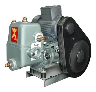
Piston pumps with electrically isolated motor drawn rocker, V-belt pulley, V-belt, membrane safety valve (type tested), poppet valve, base plate and belt guard.
