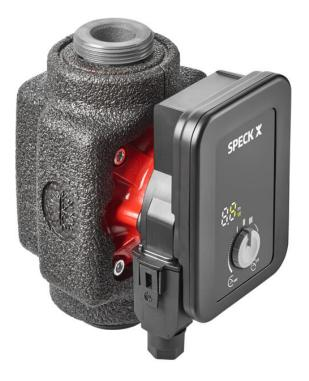
High-efficiency wet rotor circulation pump with blocking-current proof synchronous motor and integrated electronic control for stepless performance adaptation. The circulation pumps include a control module with LED display for simply adjusting the dynamic head and the control mode.
