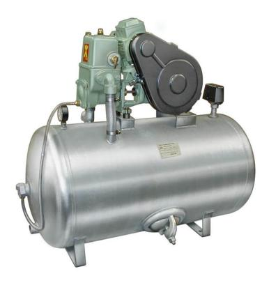
The pump, which is assembled on site, is type tested and consists of the following parts: Büffel piston pump with built in membrane safety valve (type tested), electric motor, galvanized pressure vessel, pressure switch programmed from 0.2 to 3.5 bar, pressure gauge, ventilation machine, completely closed belt guard made from plastic for your safety. A motor protection switch must be provided on site.
