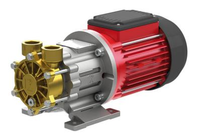
These non-self-priming regenerative turbine pumps with magnetic coupling are characterised by high pressure at low flow rates and a compact construction. Thanks to the magnetic coupling they are leakage and maintenance-free. They can be applied in circuits for liquids not containing solid matter, for example in cooling circuits or in temperature control units, among others.
