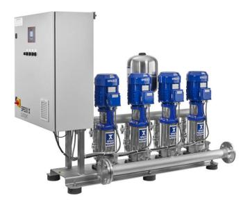
Booster units from the Multicell range are equipped with between two and six pumps, according to requirements. The fully automatic booster units are compact, have a low noise level and are supplied wired ready for connection and with the pipes in place. All units come with a fully automatic pump control. The booster unit is fitted with variable speed adjustment.
