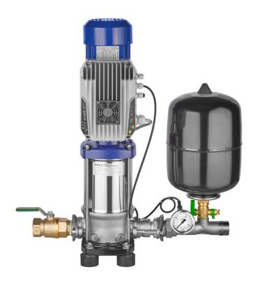
Proven quality from SPECK Pumpen. The units are turned on and off automatically via a pressure transmitter on the discharge side. An 8 I diaphragm pressure accumulator is mounted in the pressure line as a control cylinder. An electronic dry runnin gprotection is also integrated. Speed regulation, including an LED display and keyboard, is carried out via a frequency converter fitted to the motor. Bluetooth monitoring via a smartphone app. Wired eady for connection with a 1.5 m cable and plug.
