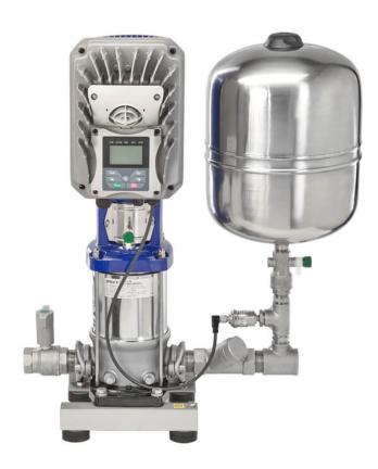
Booster units from the Aquacell range contain a non-self-priming, staged centrifugal pump. The fully automatic booster units are compact, have a low noise level and are supplied wired ready for connection and with the pipes in place. All units come with a fully automatic pump control. The booster unit is fitted with variable speed adjustment.
