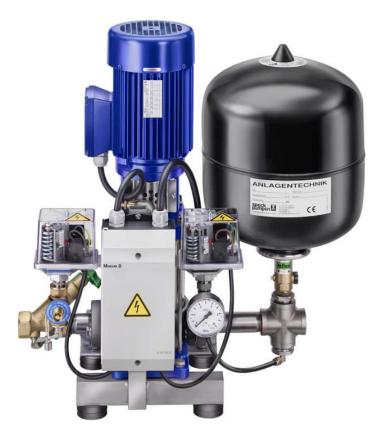
Booster units from the Aquacell range contain a non-self-priming, staged centrifugal pump. The fully automatic booster units are compact, have a low noise level and are supplied wired ready for connection and with the pipes in place. All units come with a fully automatic pump control.
