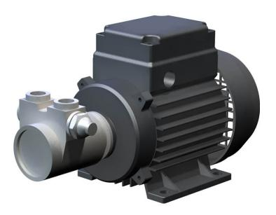
These self-priming rotary vane pumps have a relatively constant flow rate at an operating pressure of up to 14 bars. An integrated overflow valve – can be set from 4 bars of excess pressure – protects sensitive unit components. These pumps can be applied, for example, in spray applications and osmosis units.
