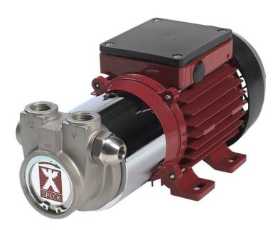
These self-priming rotary vane pumps with magnetic coupling have a relatively constant flow rate at an operating pressure of up to 14 bars. An integrated overflow valve – can be set from 4 bars of excess pressure – protects sensitive unit components. These pumps can be applied, for example, in spray applications and osmosis units.
