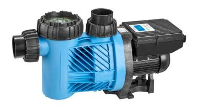
With its motor concept, the BADU Eco Flex becomes an energy-conscious circulation pump for large pools. In the private and public sector, it can be used for pools with a size of 30 - 200 m³. A plug-in converter mounted on the motor allows a space-saving design. The plain text display allows user-friendly programming. The simple programming via touchpad as well as a multitude of analogue and digital interfaces make the application even more effortless.
