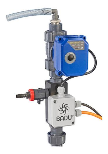
Manual venting is no longer necessary. This process is now as fully automatic as the monitoring because the unit is connected directly to the pump control. This means that if air has accumulated in the pump via the suction line, the dry running protection switches it off and opens the vent valve so that the air can escape. When the sensor comes into contact with water again, the valve is closed after an adjustable delay time and the pump restarts.
