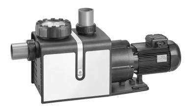
The first sealless swimming pool pump with magnetic coupling instead of a mechanical seal. The motor performance is transmitted, contactless and wear-free, via a magnetic coupling and through the can to the impeller. The pump has a maintenance-free construction and cools itself by means of a unique circulation system.
