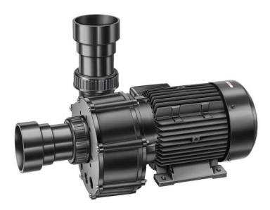
The BADU 21 range pumps are designed for the specific demands of bath tubs, whirlpools, counter swim units and cleaning devices. All models in this range are non-self-priming circulation pumps, which cannot handle air. These pumps are to be installed below the water level in order for the pool water to drain independantly.
