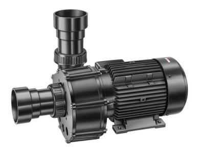
The BADU 21 range pumps are designed for the specific demands of bath tubs, whirlpools, counter swim units and cleaning devices. All models in this range are non-self-priming circulation pumps, which cannot handle air. These pumps are to be installed below the water level in order for the pool water to drain independently.
