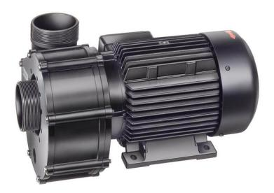
The BADU 21 range pumps are designed for the specific demands of bath tubs, whirlpools, counter swim units and cleaning devices. All models in this range are non-self-priming circulation pumps, which cannot handle air. These pumps are to be installed below the water level in order for the pool water to drain independently.
