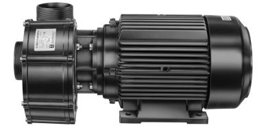
Due to the AK design and the special mechanical seal SIC/SIC Viton, the pump can also be used for higher salt concentrations than 0.5 %. The leakage possible in brine applications can drip down via the intermediate lantern and does not migrate into the motor bearing on the A-side. This prevents premature failure of the pump.
