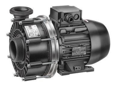
The BADU 21 range pumps are designed for the specific demands of bath tubs, whirlpools, counter swim units and cleaning devices. All models in this range are non-self-priming circulation pumps, which cannot handle air. These pumps are to be installed below the water level in order for the pool water to drain independantly.
