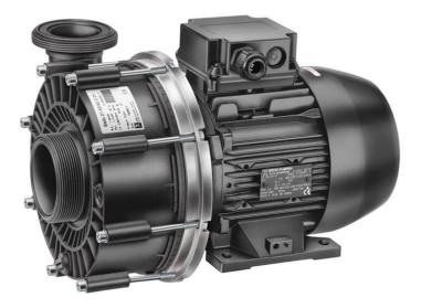
The BADU 21 range pumps are designed for the specific demands of bath tubs, whirlpools, counter swim units and cleaning devices. All models in this range are non-self-priming circulation pumps, which cannot handle air. These pumps are to be installed below the water level in order for the pool water to drain independently.
