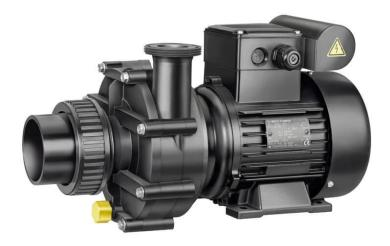
The BADU 21 range pumps are designed for the specific demands of bath tubs, whirlpools, counter swim units and cleaning devices. All models in this range are non-self-priming circulation pumps, which cannot handle air. These pumps are to be installed below the water level in order for the pool water to drain independently.
