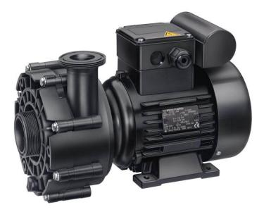
The BADU 21 range pumps are designed for the specific demands of bath tubs, whirlpools, counter swim units and cleaning devices. All models in this range are non-self-priming circulation pumps, which cannot handle air. These pumps are to be installed below the water level in order for the pool water to drain independently.
