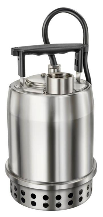
The stainless steel submersible pumps from the TOP 71 range are especially suitable for handling clean, clouded or slightly contaminated water, for example swimming pool water, ground water, rainwater and clarified sludge. All wetted parts are made from stainless steel 1.4301. The non-return valve is included in delivery.
